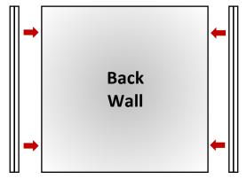
Stand the Back wall upright. Insert the Corner Connectors. (This can be done by laying the Back Wall flat, but it must be on a soft surface to avoid scratching the plastic surface)
