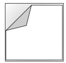
Rule #2: DO NOT remove the protective film until you are ready to insert the part into the Corner Connectors. If needed, lay plastic on soft surfaces only!
