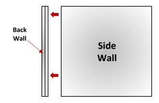
Insert the Side Walls into the Back Wall with Corner Connectors.
